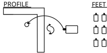
Turn the Base upside down and fix it on a flat surface. Then, mount the feet in the mounting package to the profile.
